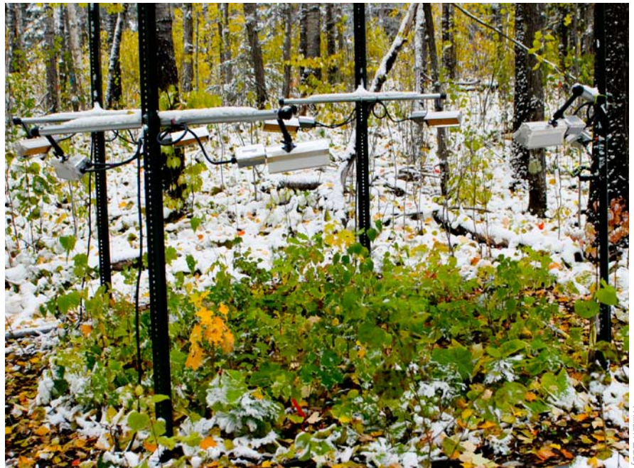
Warming equipment melts an early-autumn dusting of snow in a forest research site.
