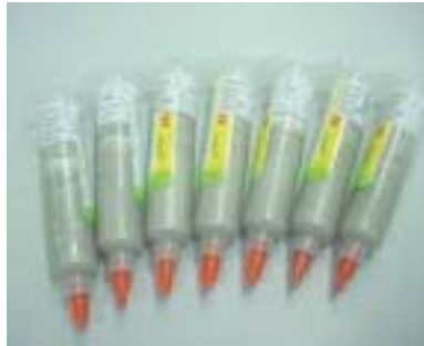
VISUAL ANALYSIS ON DIE ATTACH PASTE WASTE: These syringes were collected from the trash bin after each shift. About 80% of the die attach paste remains per syringe.
